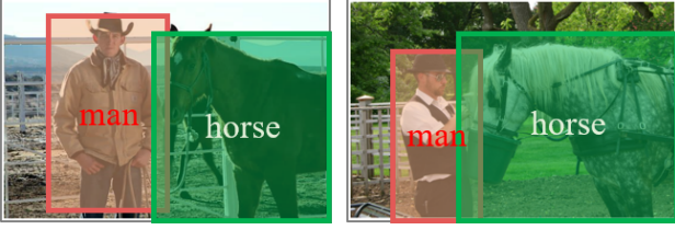
Fig. 6. Schematic diagram of object detection. The use of object detection alone essentially cannot aid in the recognition of visual relationships. The interaction of features between different objects is crucial to the recognition of relationships.
